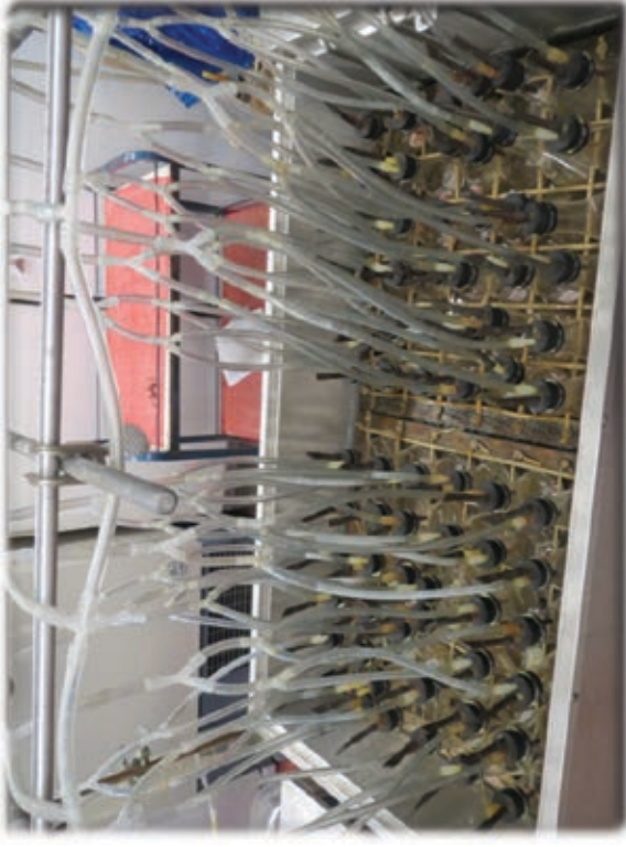
Tilley-Terry “artificial rumen” batch in vitro system
